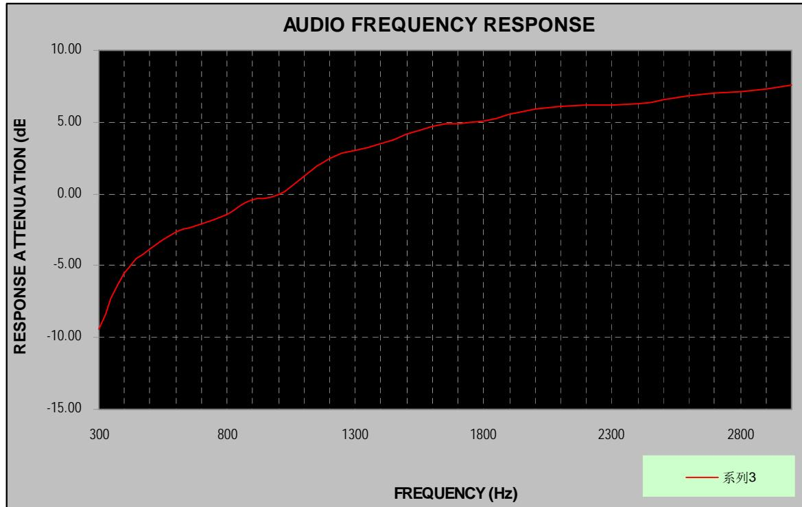
**Audio Frequency Low Pass Filter Response****Analog Modulation:**
