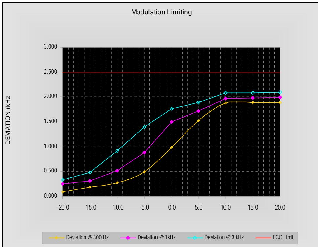
Carrier Frequency: 156.000 MHz, Channel Separation=12.5 kHz, Low Power
