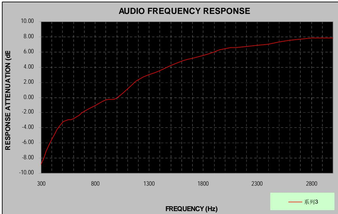
Carrier Frequency: 156.000 MHz, Channel Separation=12.5 kHz, Low Power
