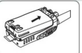
To remove the battery pack, lift the safety lock and pull the battery pack away from the radio.
