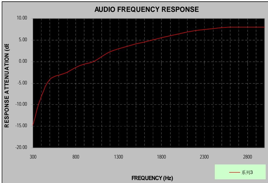
Carrier Frequency: 450.0125 MHz, Channel Separation=12.5 kHz, High Power
