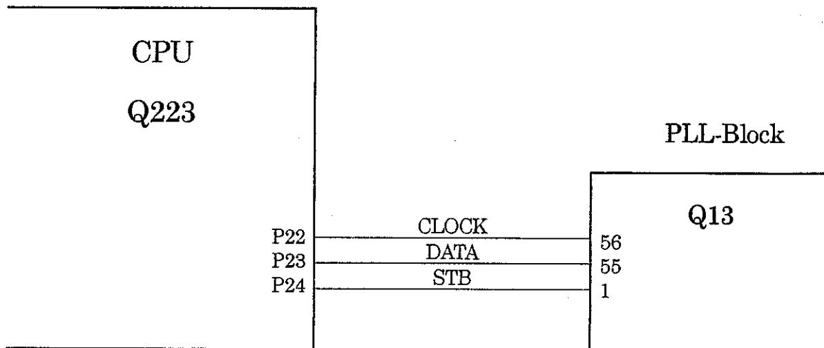
\* P22(CLOCK), P23(DATA), P24(STB) of CPU(Q223) are sent out in serial form to control 12bit programmable reference divider and 17bit programmable devider.
