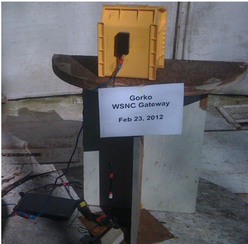
Test Setup for Spurious Radiated Emissions (Horizontal)
