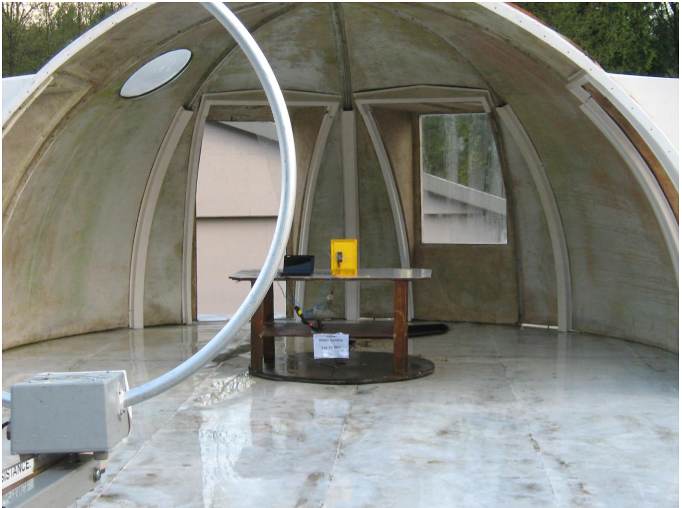
Test Setup for Spurious Radiated Emissions Frequencies below 30 MHz.
