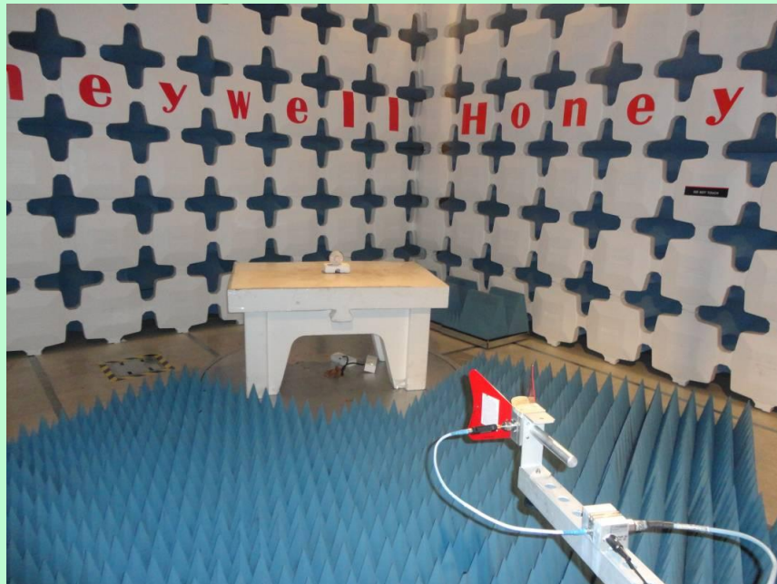
Radiated Emission Setup –1 GHz to 10 GHz [ Horizontal Polarization ]
