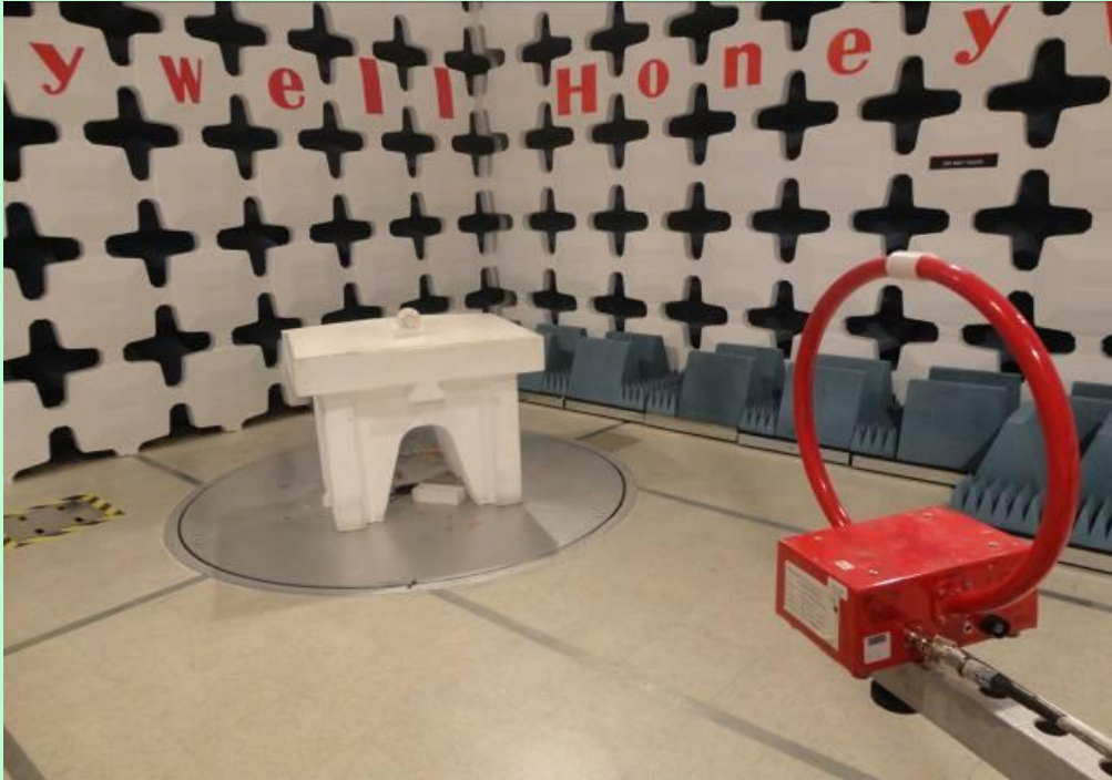
Radiated Emission Setup – 9 KHz to 30 MHz [ Parallel ]
