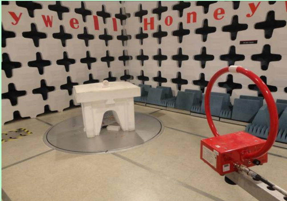
Radiated Emission Setup – 9 KHz to 30 MHz [ Parallel ]
