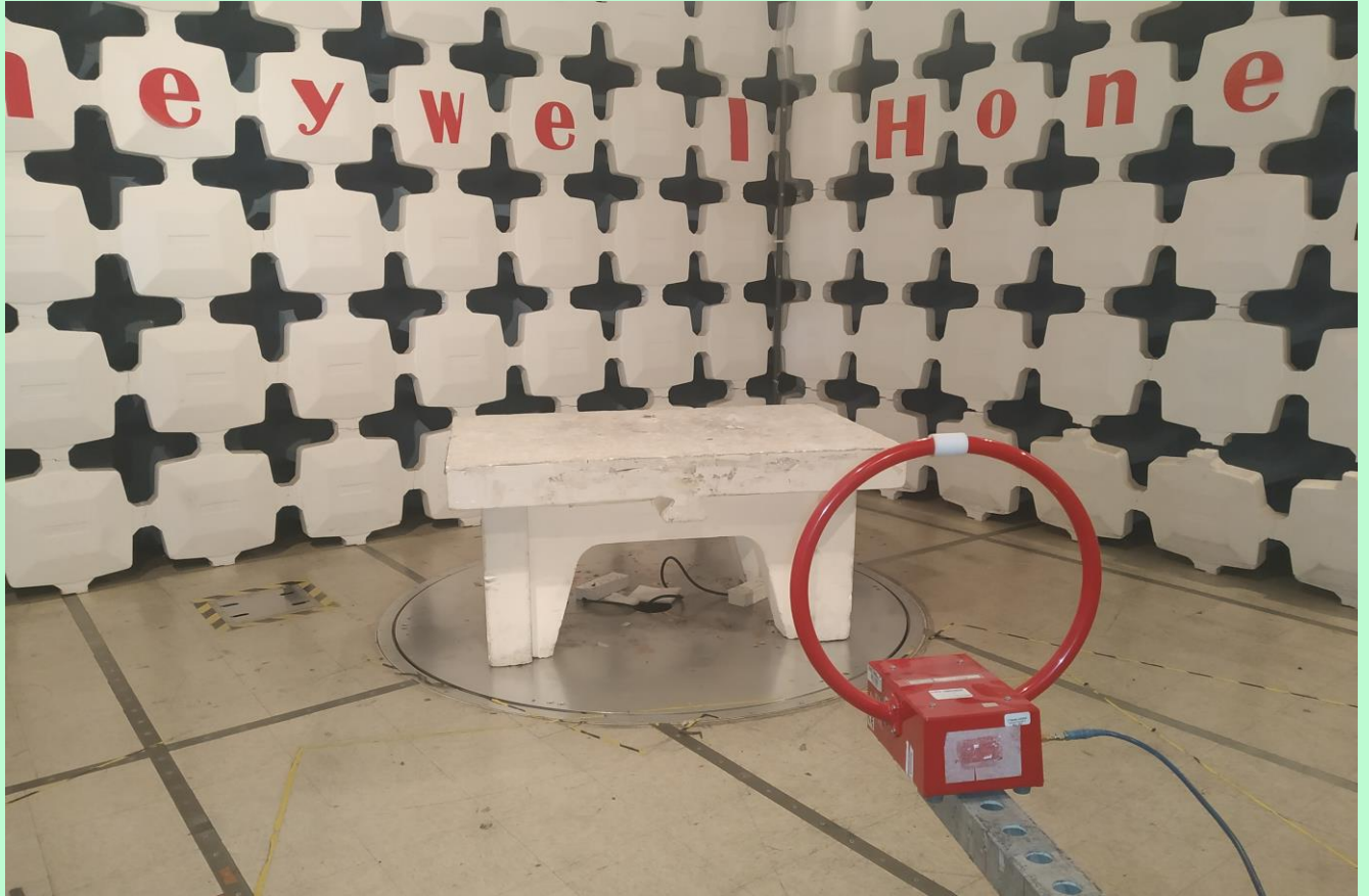
Radiated Emission Setup – 9 KHz to 30 MHz [ Parallel ]
