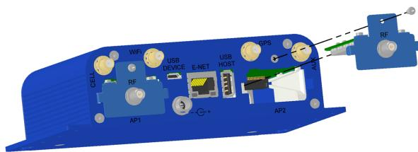
3. Unscrew and remove the slot cover from the device. Save the removed screw for the next step. Slide the card into the open slot. You should feel the card connector seat in the internal connector.
