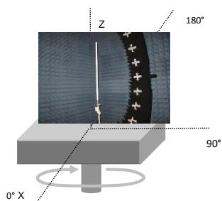
Elevation Cut (Phi Axis = 0°)
