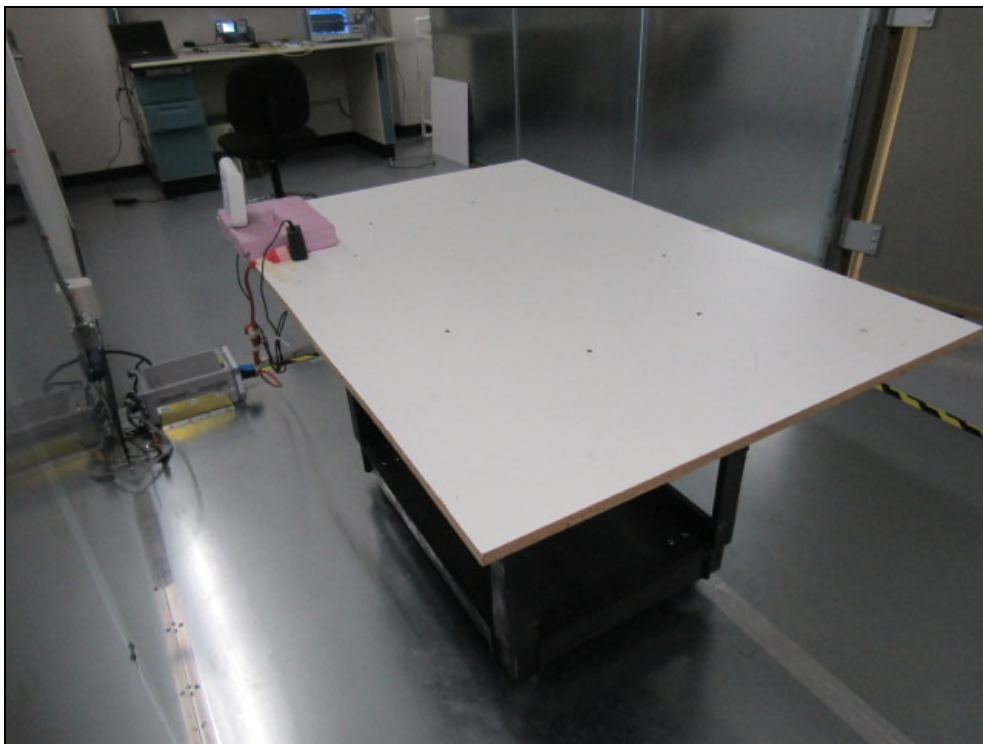
Figure 2: Powerline Conducted Emissions - Back
