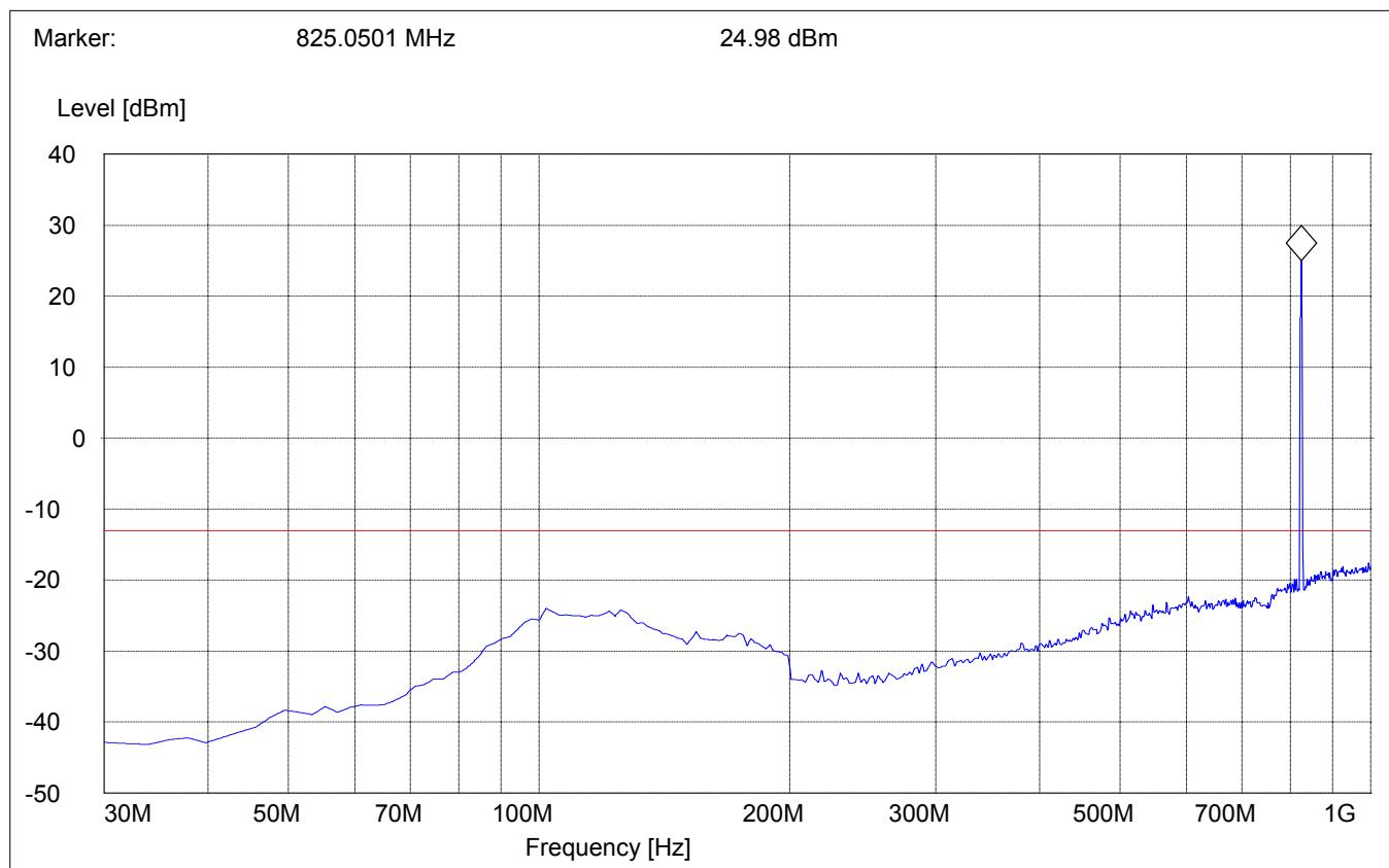
**RADIATED SPURIOUS EMISSIONS (GSM-850)****Tx @ 824.2MHz: 1GHz – 1.58GHz**
