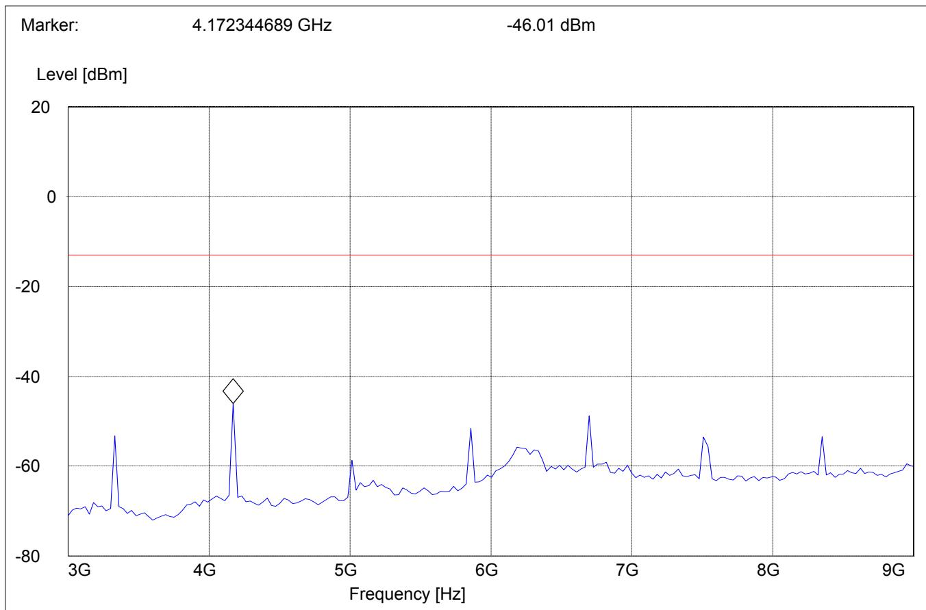
**RADIATED SPURIOUS EMISSIONS (GSM-850)****Tx @ 848.8MHz: 1GHz – 1.58GHz**
