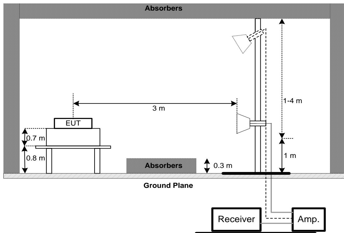
(C) For Radiated Emissions Below 30MHz
