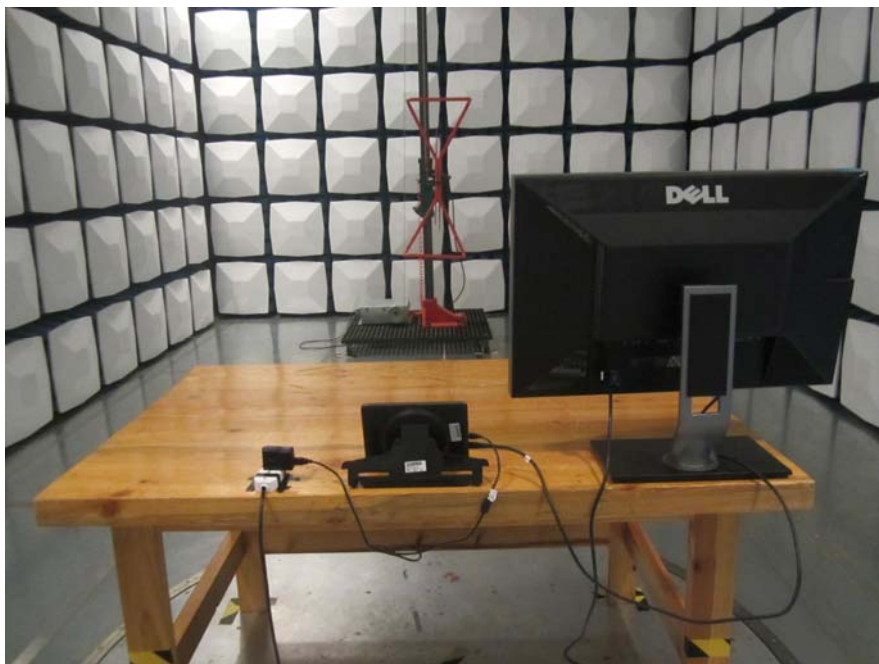
Radiated Emission - Rear View (Below 1GHz)
