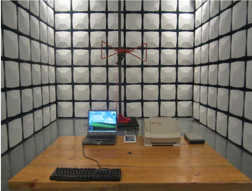
Radiated Emission Below 1GHz -Front View (USB Downloading)
