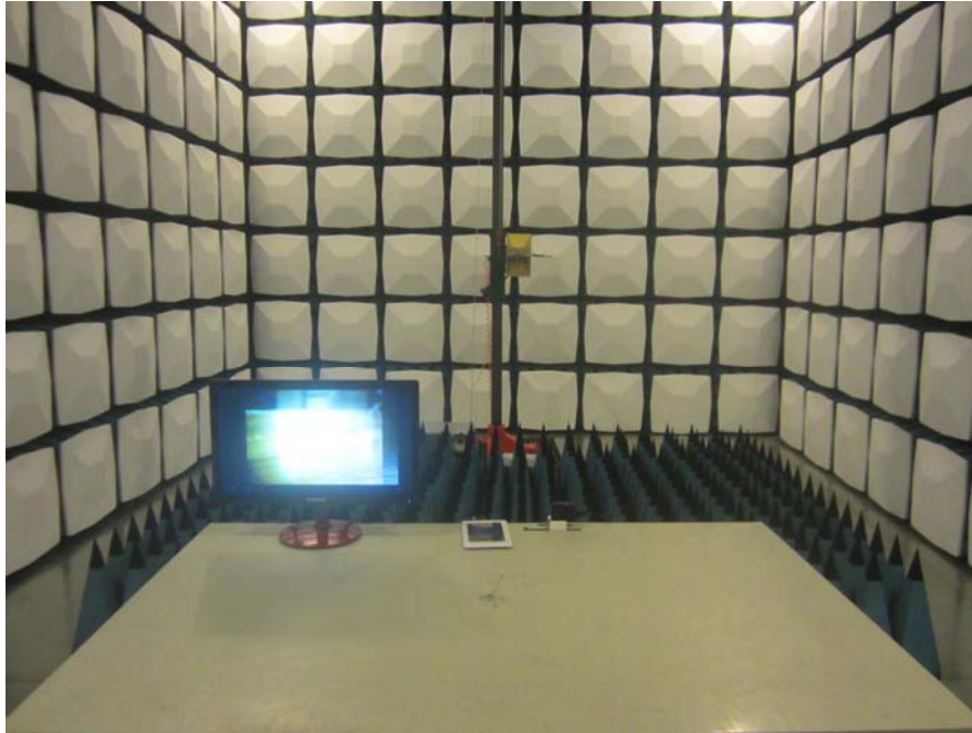
Radiated Emission Above 1GHz -Front View (HDMI Playing)
