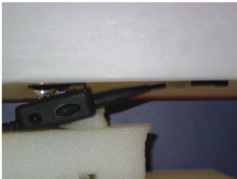
Test Position Audio Accessory D Body 0 mm Gap
