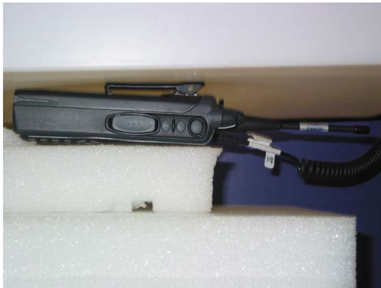
Test Position Handset Body 0 mm Gap
