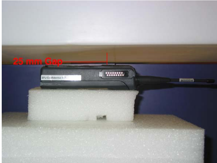
Test Position Handset Face 25 mm Gap
