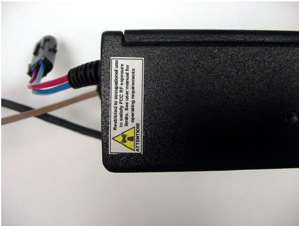
Radio side showing RF safety label
