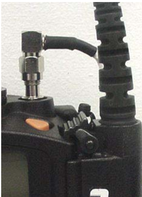
Front View of Antenna Termination
