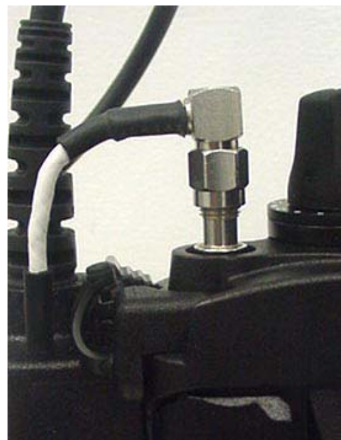
Back View of Antenna Termination
