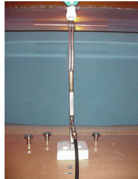
450MHz Dipole Setup
