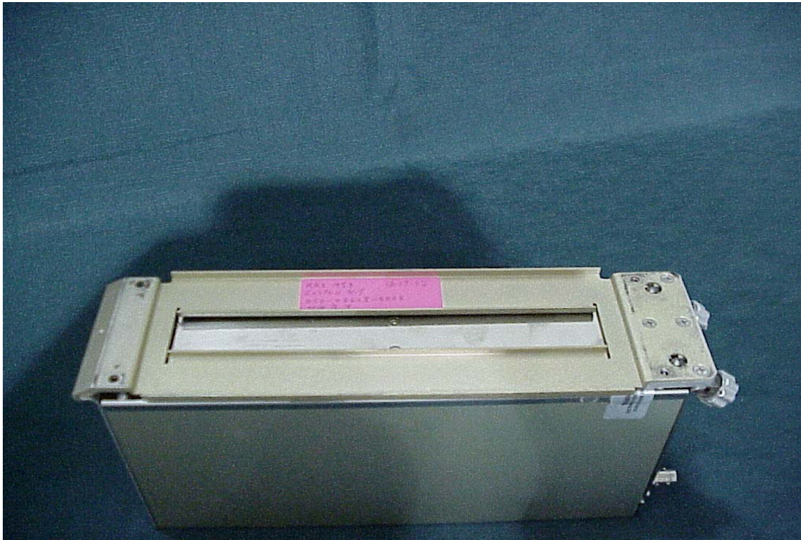
KRX 1053 Receiver Exciter (mounting tray, bottom)
