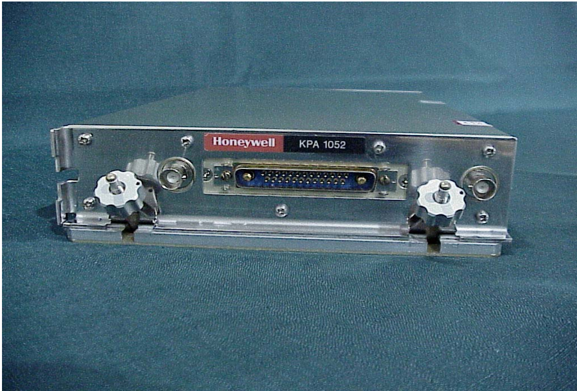
KPA 1052 Power Amplifier (front view)
