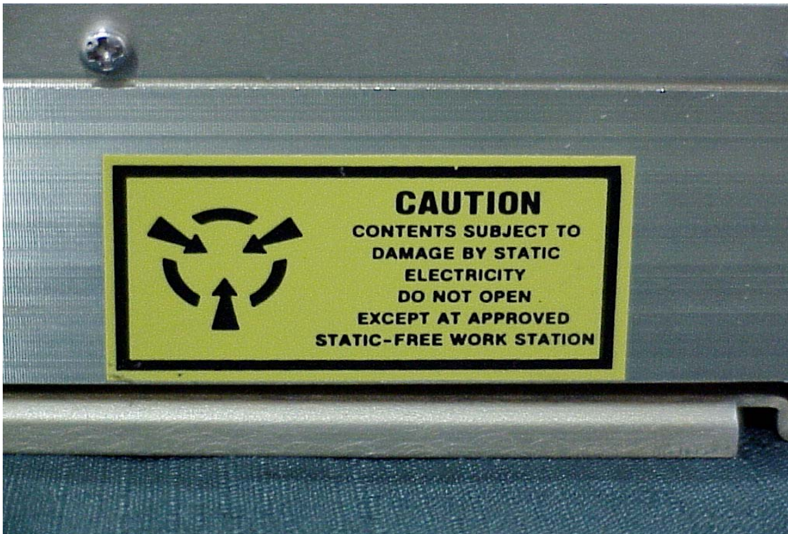
KPA 1052 Power Amplifier (electrostatic warning tag)
