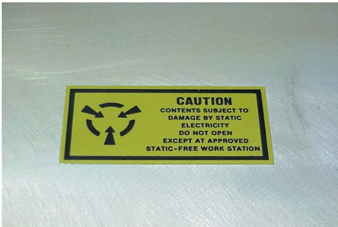
KAC 1052 Antenna Coupler (electrostatic warning tag)
