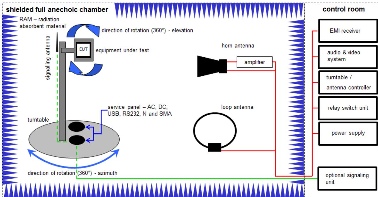
Measurement distance: tri-log antenna and horn antenna 3 meter; loop antenna 3 meter / 1 meter
