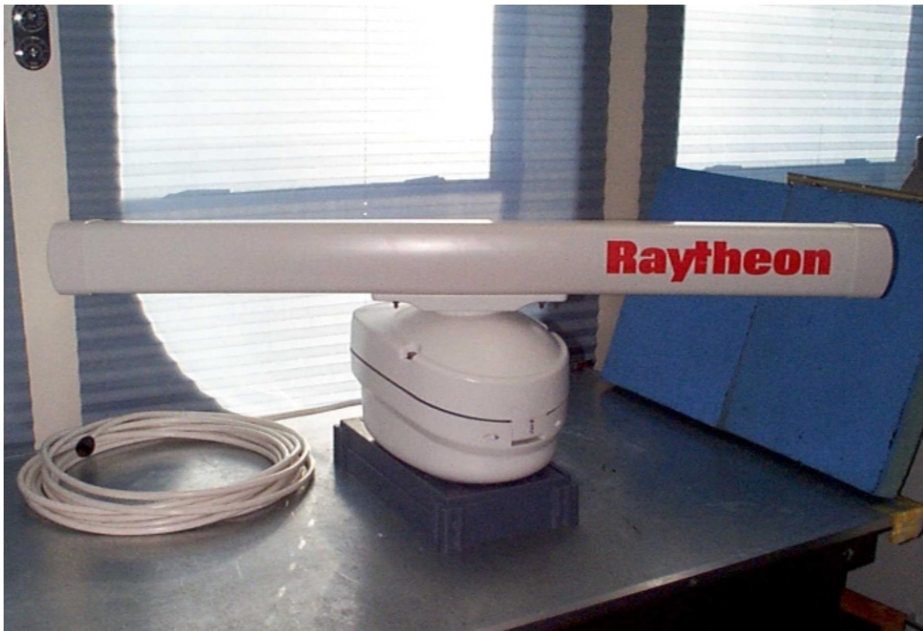
10kW, 48" Open Array Scanner Unit
