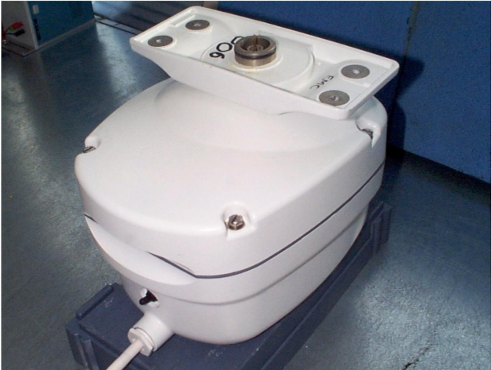
10kW, 48" Open Array Scanner Unit
