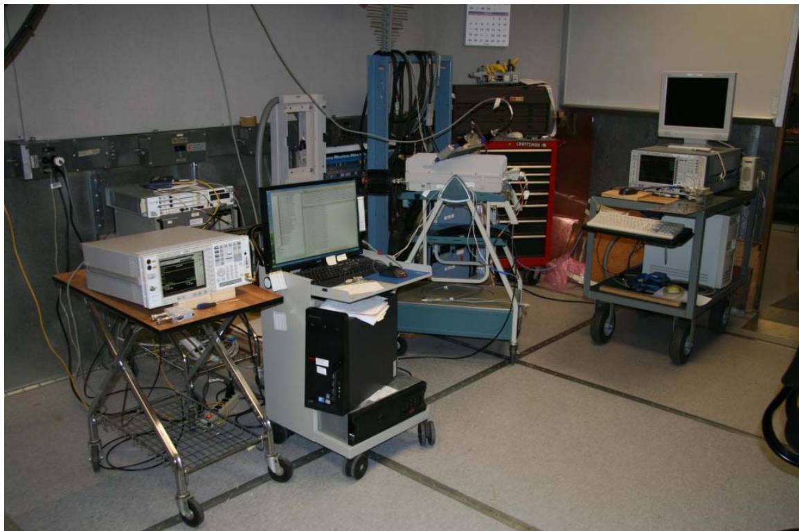
**TEST: Measurement of Radiated Spurious Emissions**
