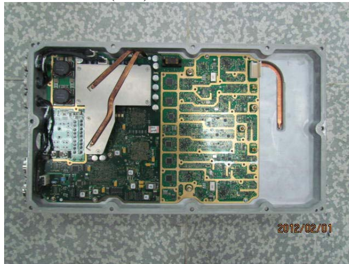
TRANSCIEVER (TRX) - BOTTOM with COVER REMOVED
