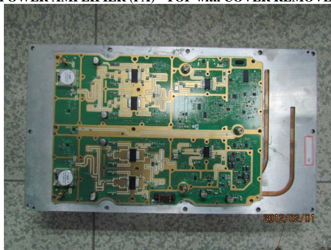
POWER AMPLIFIER (PA) - TOP with COVER REMOVED
