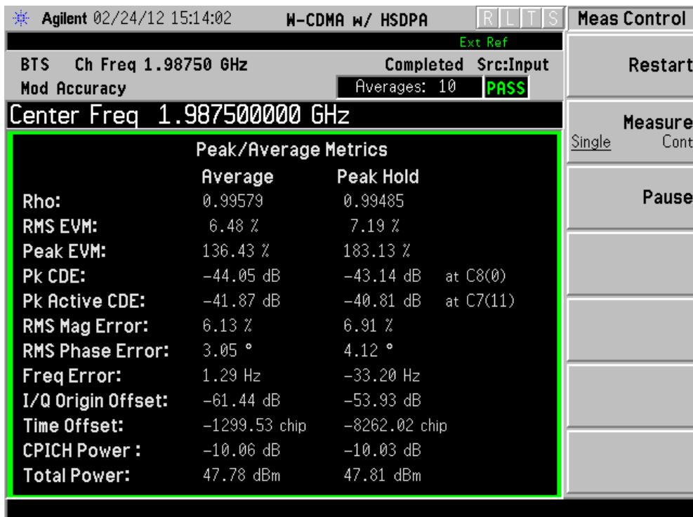
**Test Modulation: TM 5-44 with 44 active channels: 30 voice + 8 HSDPA (High Speed Downlink Packet Access) channels + 6 control (16QAM). Limit: EVM RMS < 12.5 %.**
