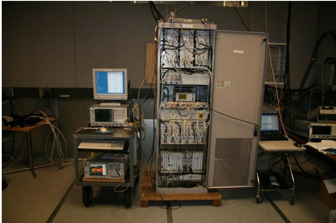
**TEST: Measurement of Radiated Spurious Emissions**
