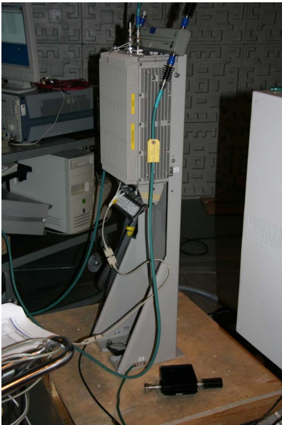
TEST: Measurement of Radiated Spurious Emissions
