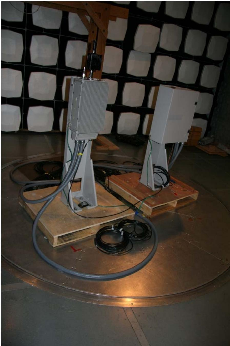
TEST: Measurement of Radiated Spurious Emissions
