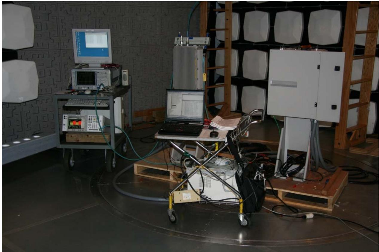
View: UMTS 9341 RRH 60W 1900MHz RF Remote Radio Head (RRH) Under Test -
