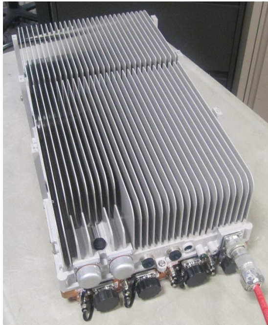
External Front View of the RRH without Solar shield
