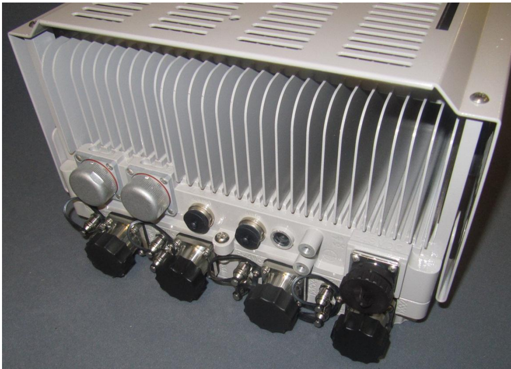
External Bottom View of the RRH
