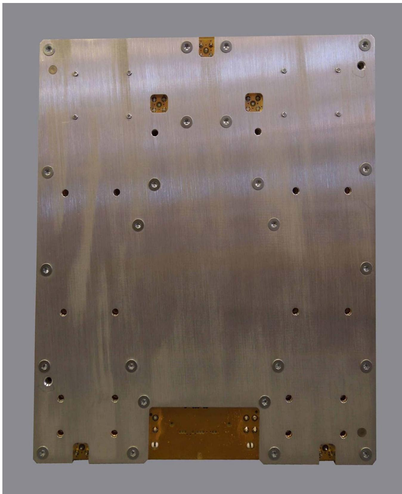
**Front Internal of PA Board with Shield**
