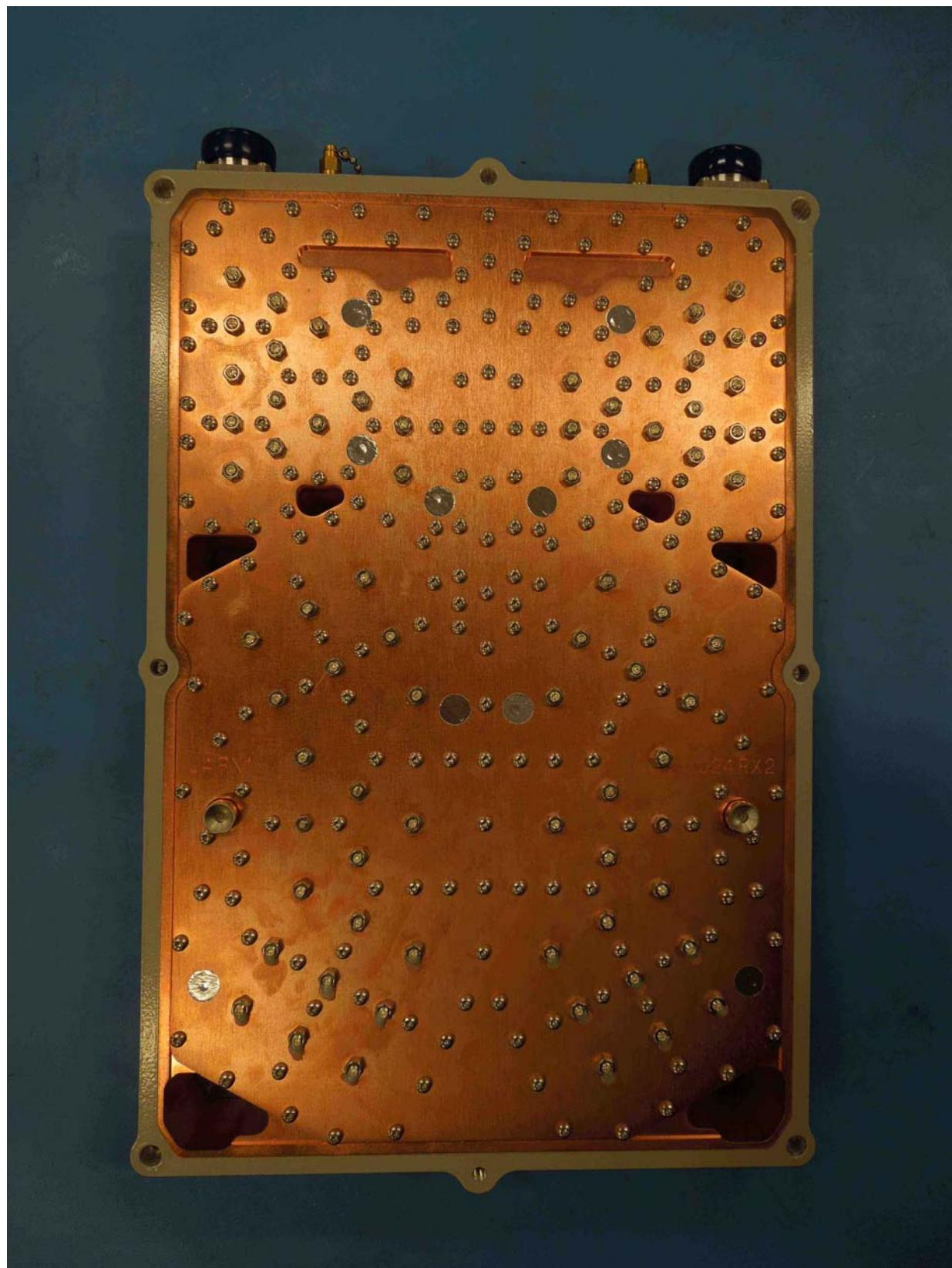
Rear Internal of Transmit Filter
