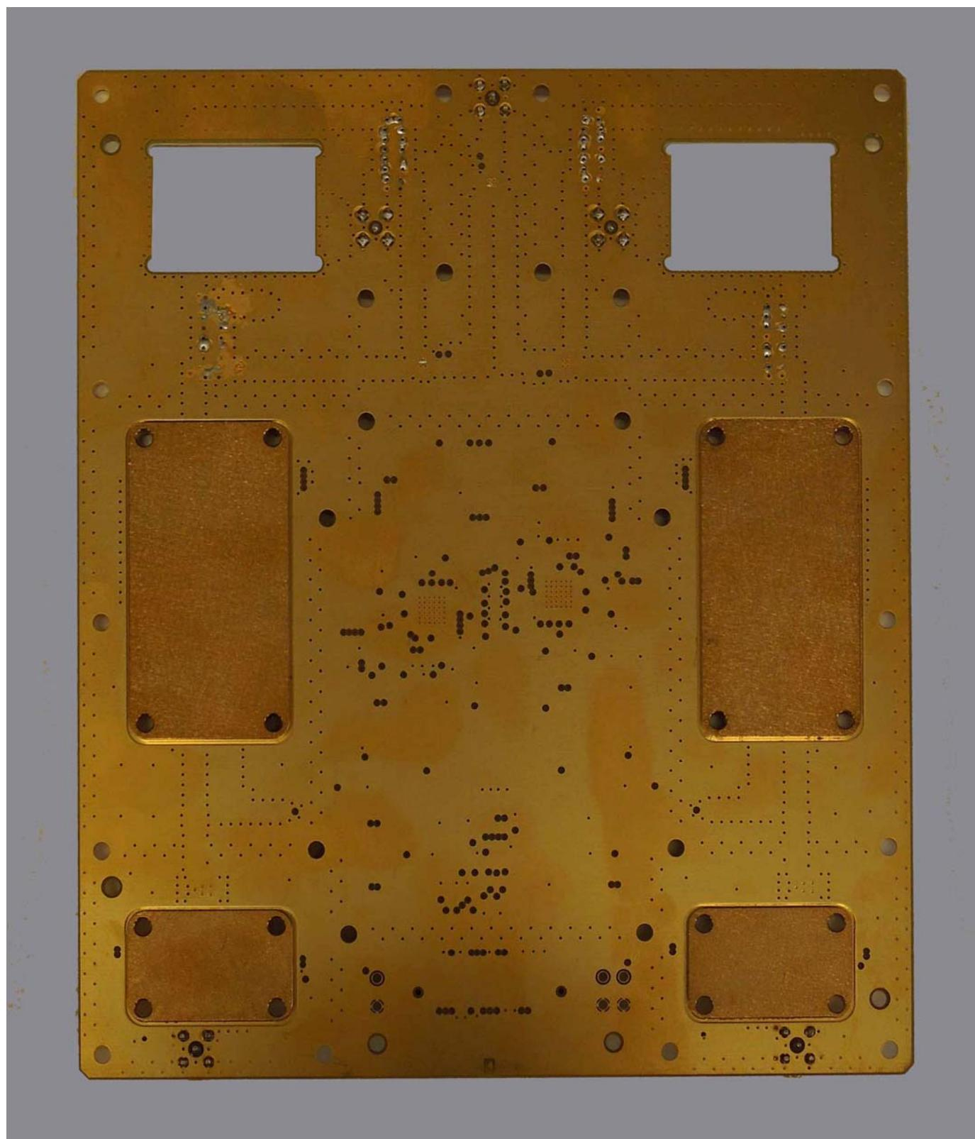
**Front Internal of PA Board with Shield**
