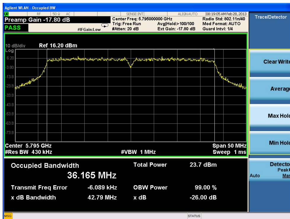
Figure 4.4.3 The Minimum 26dB Emission Bandwidth Measured (42.79MHz) for 802.11n (HT40-2Tx-2S) Carrier at Ch 159/5795MHz, 18dBm, OFDM/SM, MCS8, Port 1.
