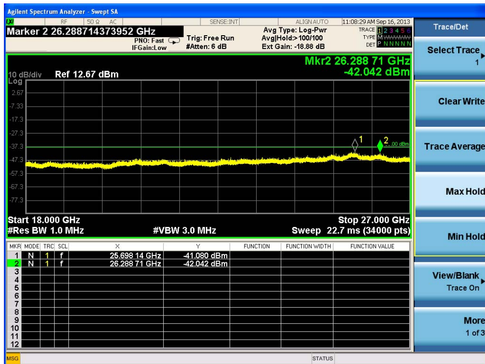
Figure 4.8.4 The Highest Out-of-Band Conducted Emissions Measured for 802.11a (20MHz-2Tx) Carrier at Channel 149/5745MHz, 18dBm, High Gain Antenna, Peak Detector, Max Hold, OFDM/CDD, 6 Mbps, Port 2.
