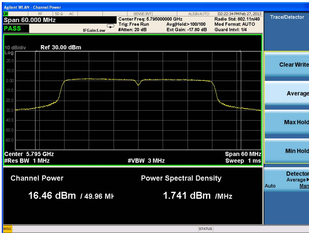
Figure 4.5.2 The Mean Output Power Measured for 802.11n (40MHz-2Tx-1S) Carrier at Channel 159/5795MHz, 18dBm, Medium Gain Antenna, OFDM/CDD, MCS0, at Two Ports. (16.50dBm+16.46dBm = 19.99dBm)
