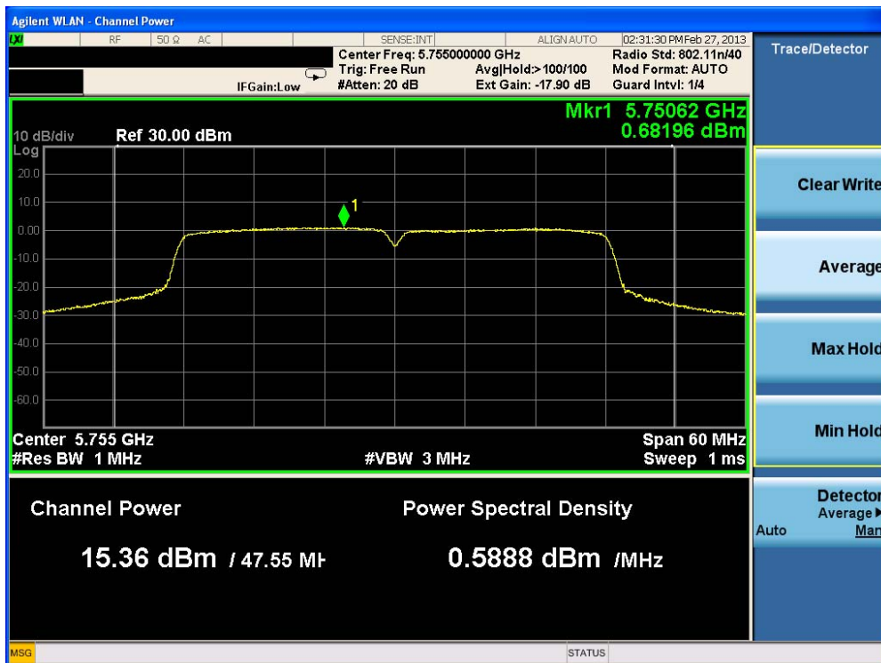
Figure 4.6.2 The PPSD for 40MHz Carriers with Minimum Margin Measured for 802.11n (40MHz-2Tx-1S) Carrier at Channel 151/5755MHz, 18dBm (High Gain Antenna), OFDM/CDD, MCS0, at Two Ports.
