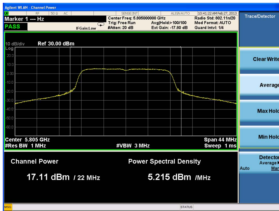
Figure 4.5.1 The Mean Output Power Measured for 802.11n (20MHz-2Tx-2S) Carrier at Channel 161/5805MHz, 18dBm, OFDM/SM, MCS8, at Two Ports. (17.17dBm+17.11dBm = 20.15dBm)
