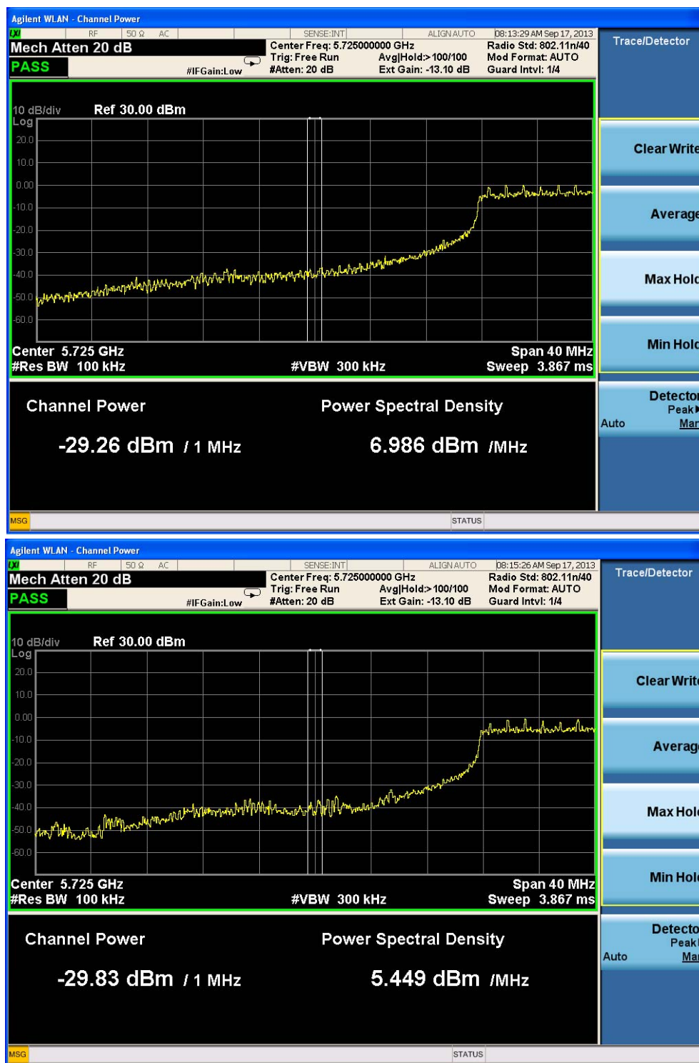
Figure 4.8.1 The Out-of-Band Emissions near Left Band Edge (5.725GHz) with Minimum Margin Measured for 802.11n (40MHz-2Tx-1S) Carrier at Channel 151/5755MHz, 18dBm (High Gain Antenna), OFDM/CDD, MCS0, at Two Ports. (-29.26dBm/MHz-29.83dBm/MHz = -26.53dBm/MHz, below -25 dBm/MHz Limit)
