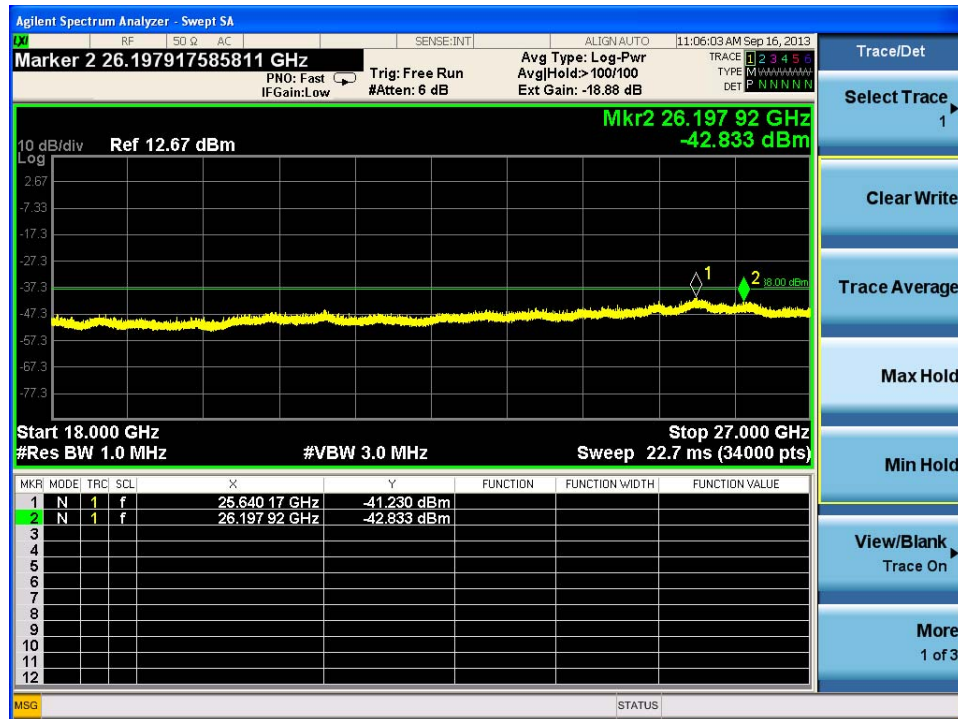
Figure 4.8.3 The Highest Out-of-Band Conducted Emissions Measured for 802.11a (20MHz-2Tx) Carrier at Channel 149/5745MHz, 18dBm, High Gain Antenna, Peak Detector, Max Hold, OFDM/CDD, 6 Mbps, Port 1.
