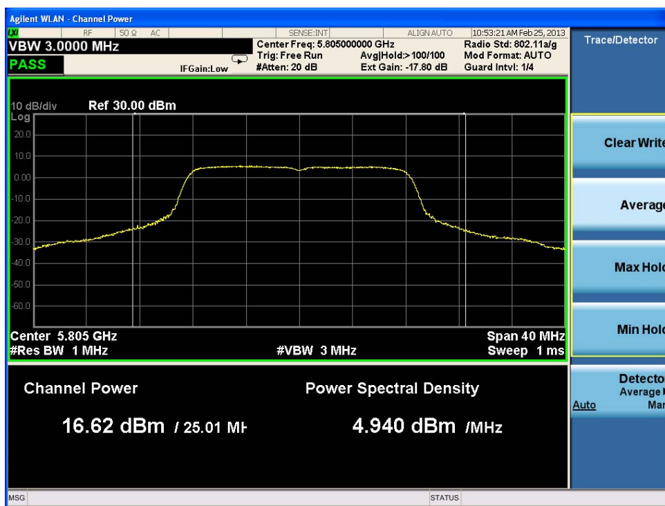
Figure 4.6.1 The PPSD for 20MHz Carriers with Minimum Margin Measured for 802.11a (20MHz-2Tx) Carrier at Channel 161/5805MHz, 18dBm, OFDM/CDD, 6Mbps, at Two Ports.
