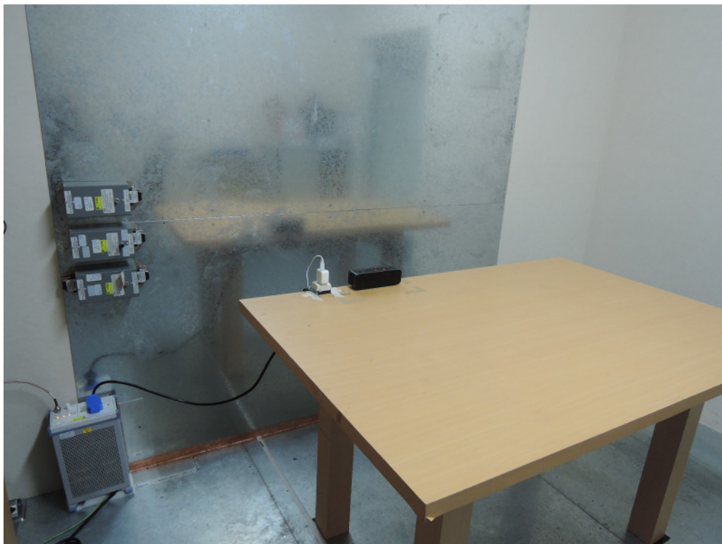
Photograph 6: Set-up for for Mains Conducted testing Front
