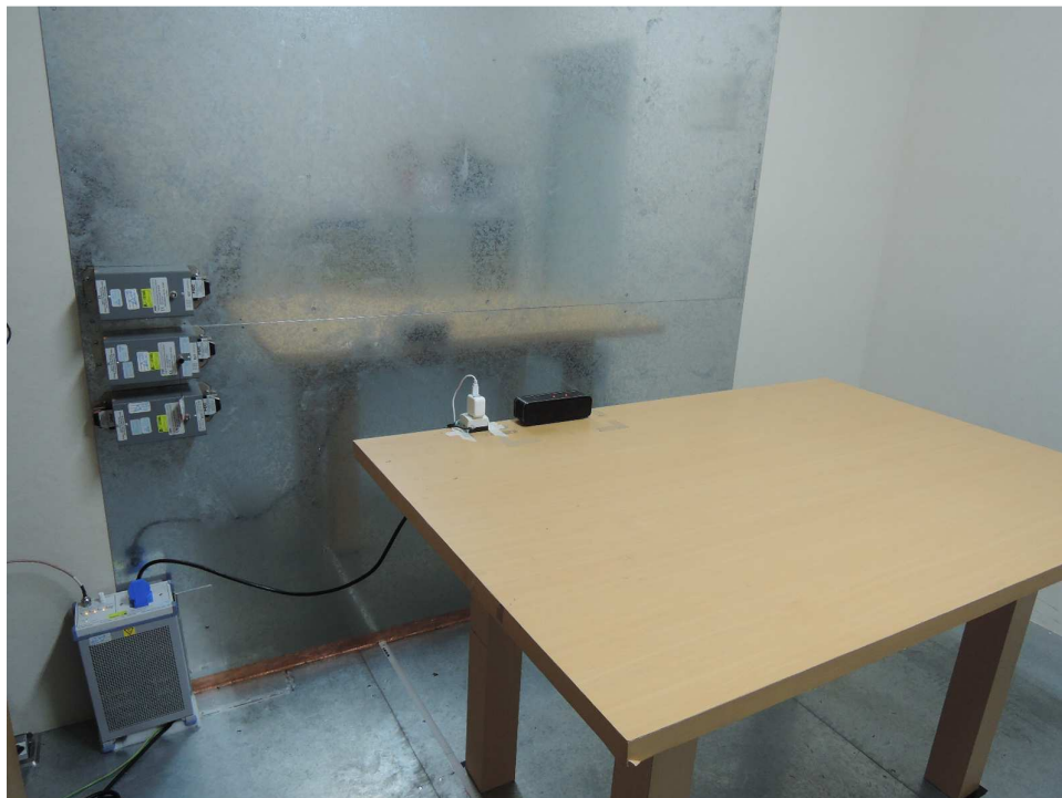
Photograph 6: Set-up for for Mains Conducted testing Front
