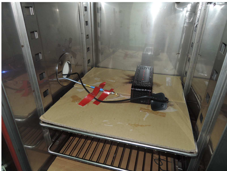
Photograph 4: Set-up for Conducted testing
