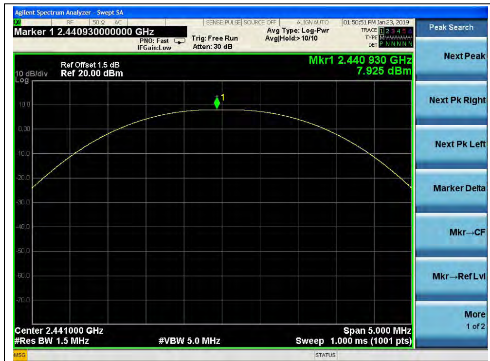
(GFSK, Channel 39, 2441MHz)
