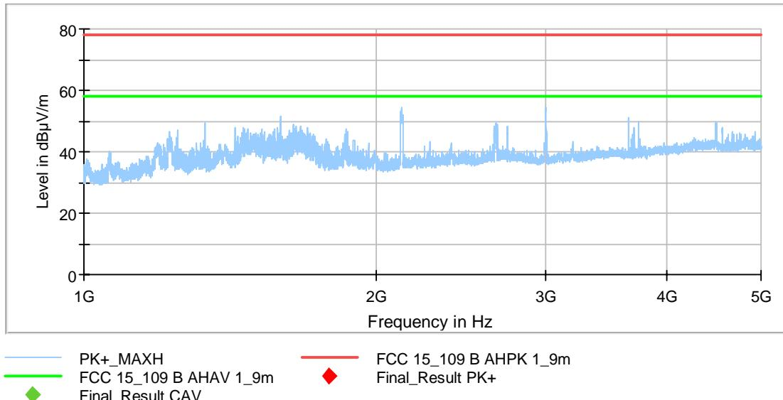
Remark\*: The measurement was carried out at a distance from 1.9 m instead of 3 m. Therefore 4 dB were added to the 3 m limit according FCC part 15.109 Class B devices. Limits extrapolated from 3 m distance to 1.9 m distance by 20 dB /decade
