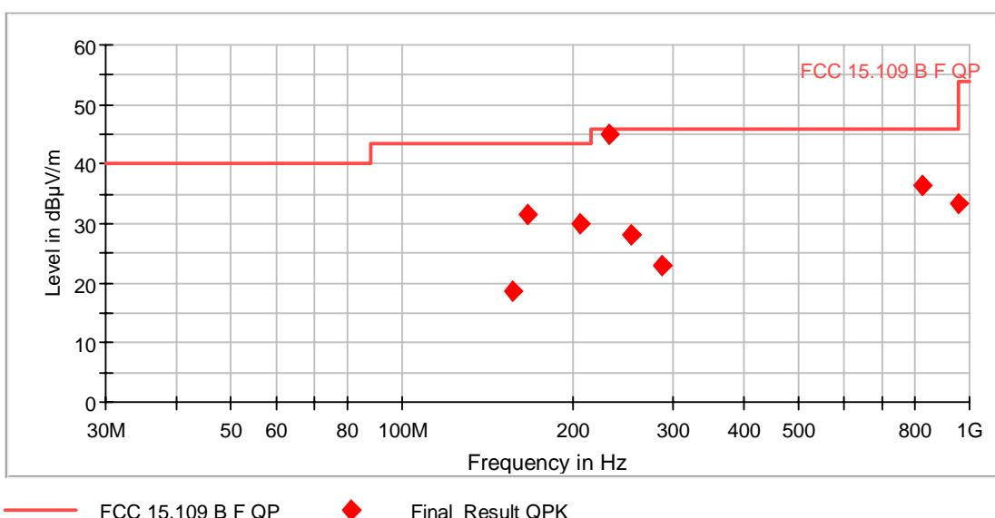
The results of the standard subsequent measurement on the open area test site are indicated in the table below. The limits as well as the measured results (levels) refer to the above mentioned standard while taking account of the specified requirements for a 3 m measuring distance.
