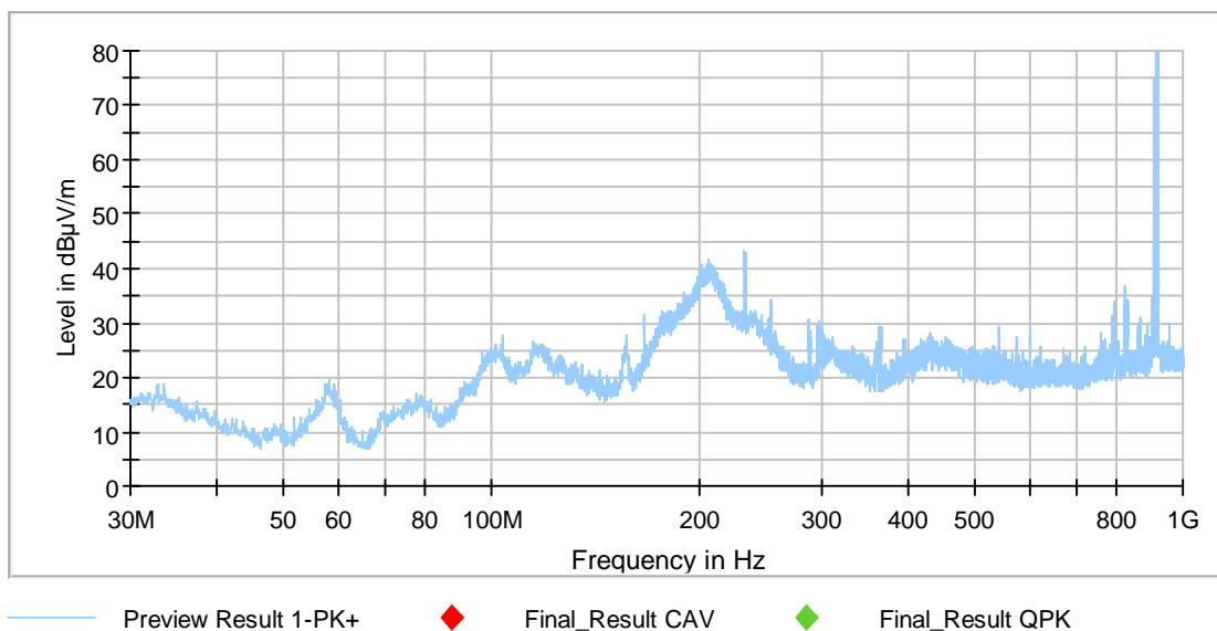
Except the wanted signal on 911.800 MHz, which is tested and documented under another rule part, the following frequencies were found during the preliminary radiated emission test:
