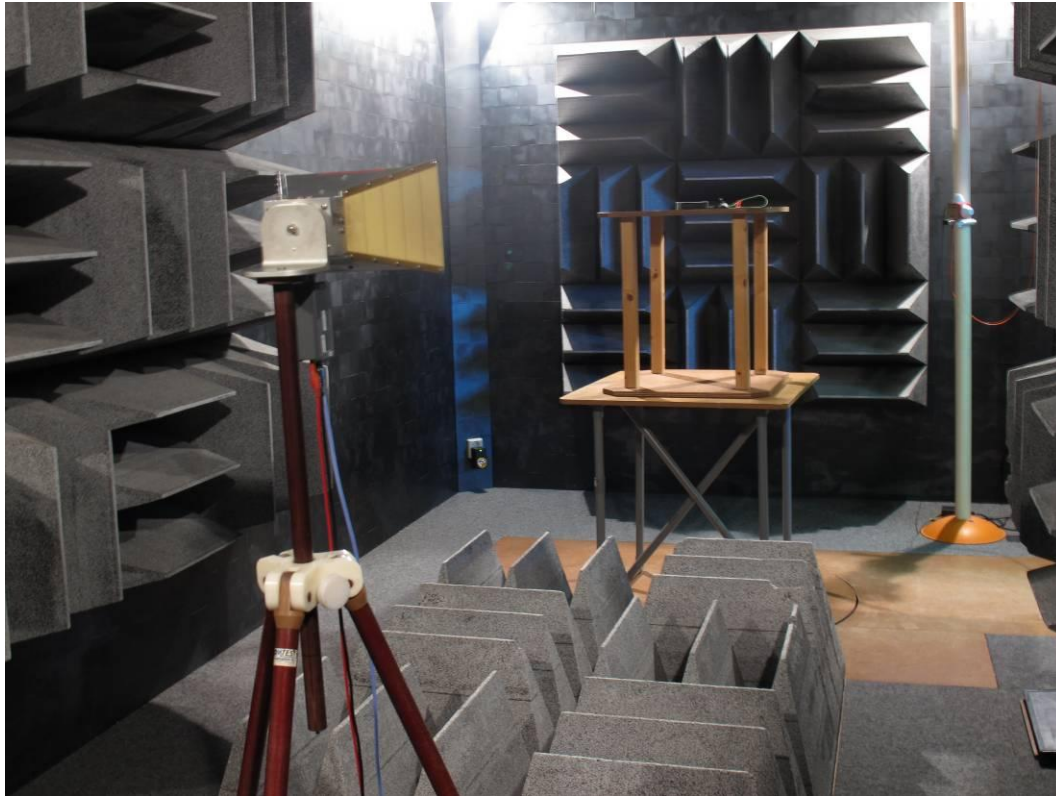
Photograph 2: Test setup radiated emissions (1 - 10 GHz)
