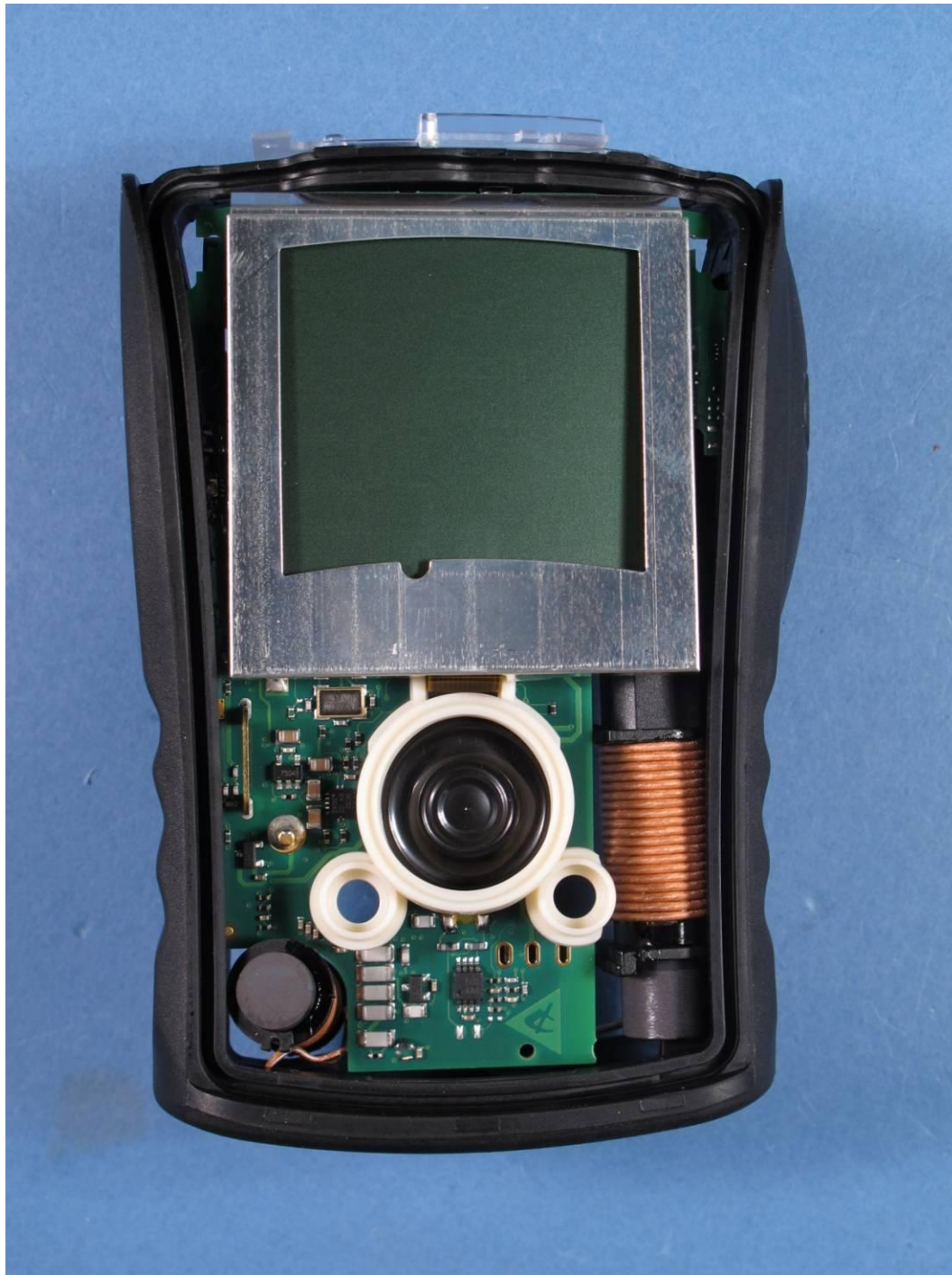
Photograph 1: - Inside view of Element Barryvox, top side
