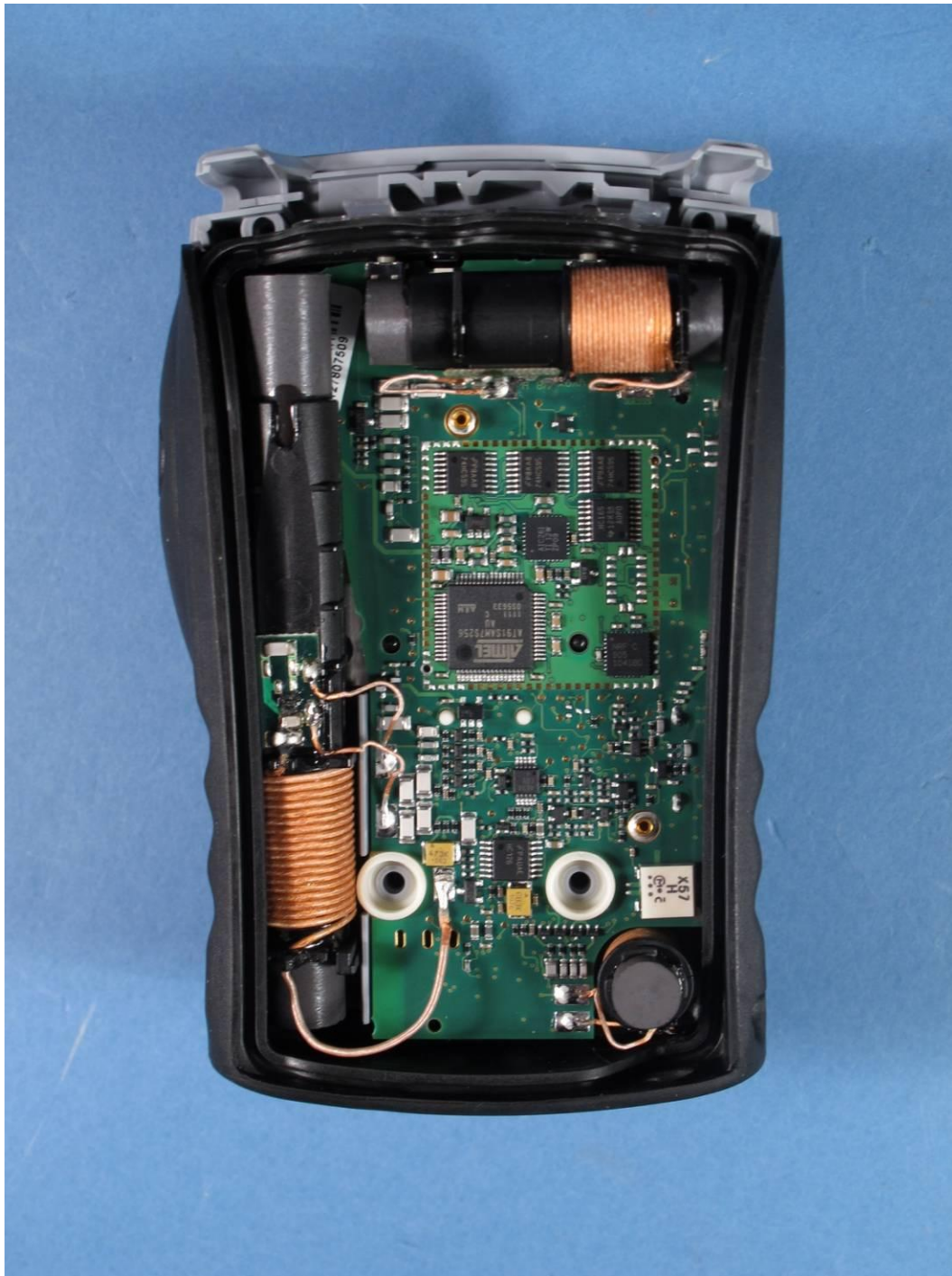
Photograph 2: - Inside view of Element Barryvox, bottom side
