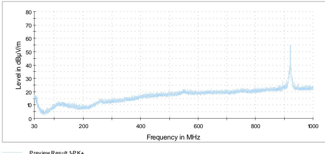
The emissions found in this frequency range are caused by the UHF transceiver of the EUT, which is will be certified under an other FCC 47 CFR Part 15 section. The measurement results for this rule section are documented under PHOENIX TESTLAB GmbH test report reference F17626E1.
