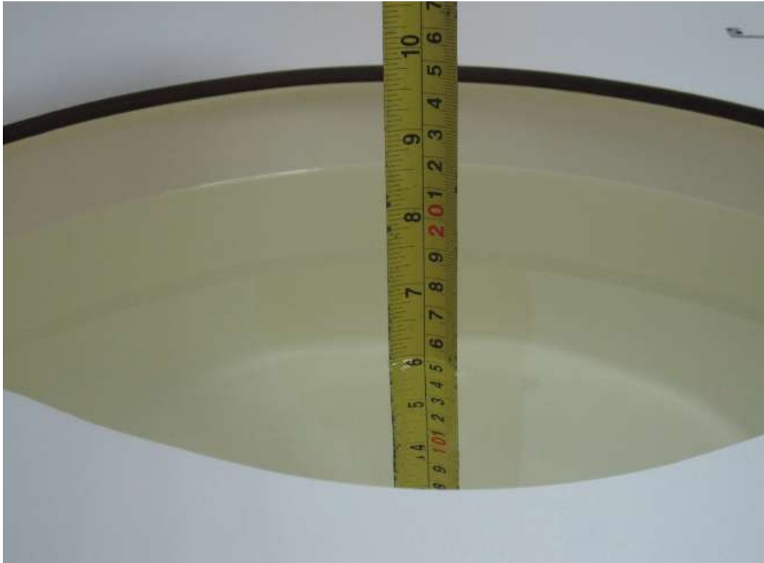
Picture C.3: Liquid depth in the flat Phantom (2600 MHz) (15.2cm deep)
