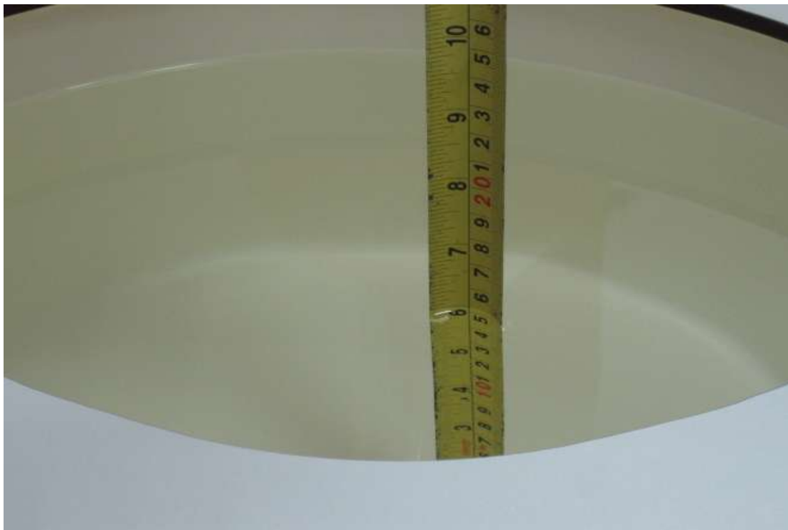
Picture C.2: Liquid depth in the flat Phantom (2450 MHz) (15.1cm deep)
