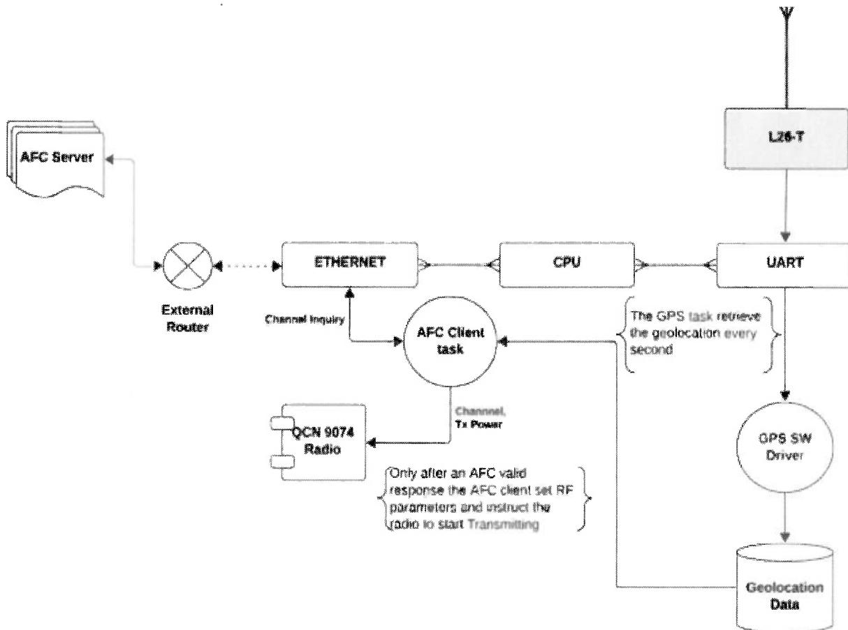
**L26-T: Quectel geolocation module communicates using NEMA protocol location, time and altitude to the CPU.**
