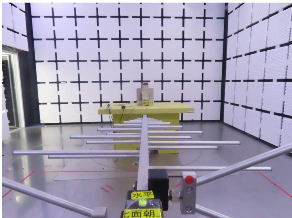
**For Antenna Configuration 1****Radiated Emissions Test Photos****Band edge & Harmonic (1 GHz to 18 GHz)**
