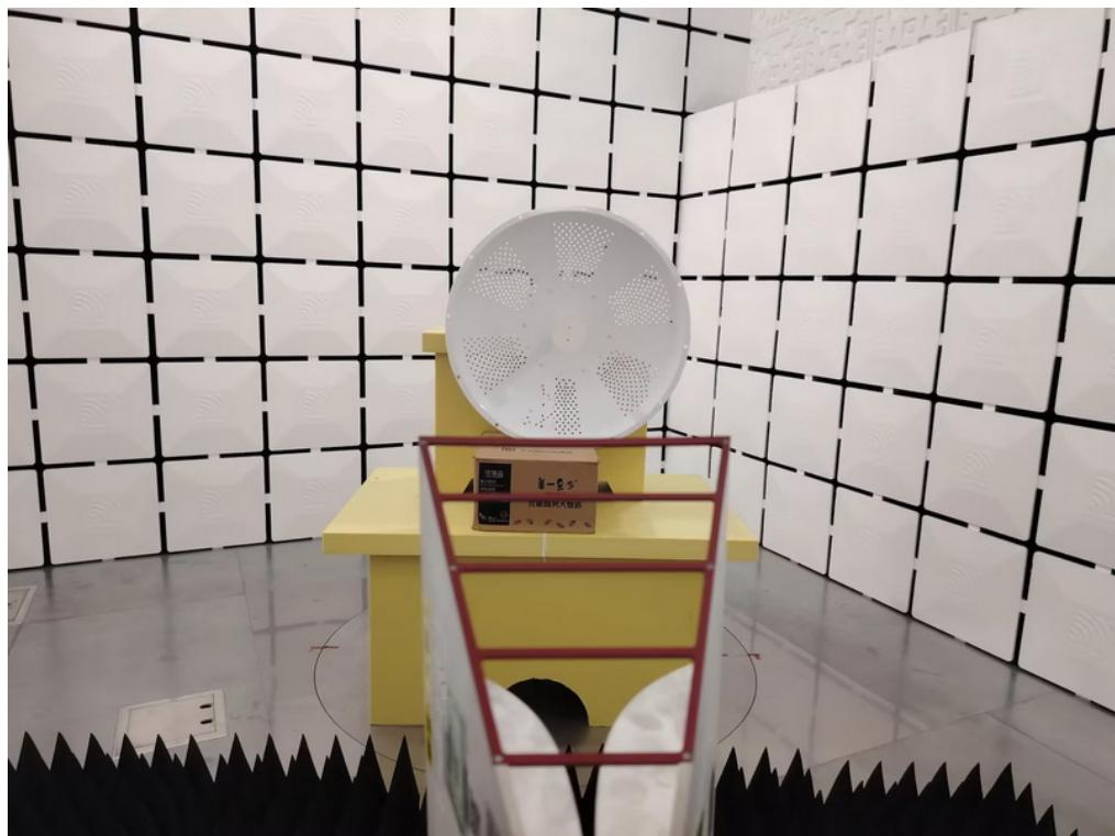
**Radiated Emissions Test Photos****Harmonic (18 GHz to 40 GHz)**
