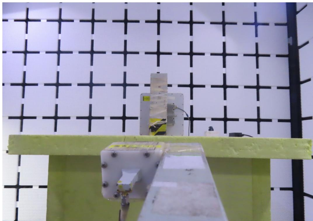
**For Antenna Configuration 2****Radiated Emissions Test Photos****Band edge & Harmonic (1 GHz to 18 GHz)**
