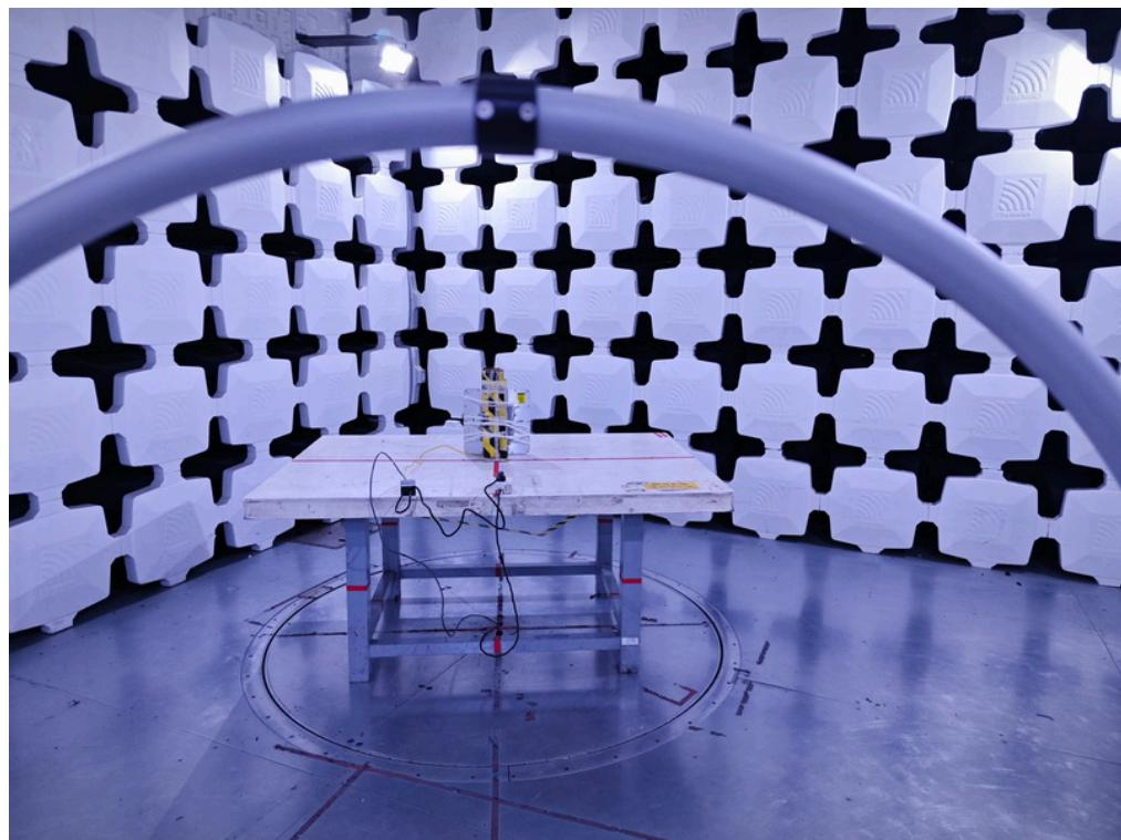
**Radiated Emissions Test Photos****30 MHz to 1 GHz**
