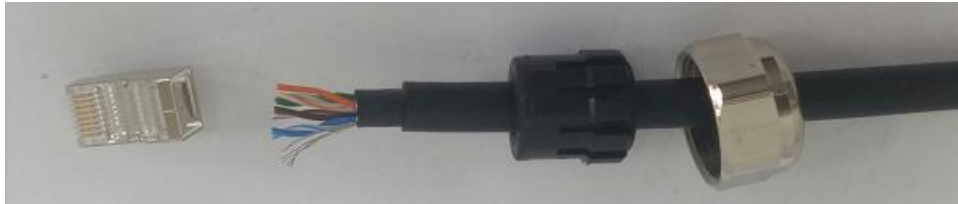
Figure 2-5: Cable preparation for Outdoor Unit
