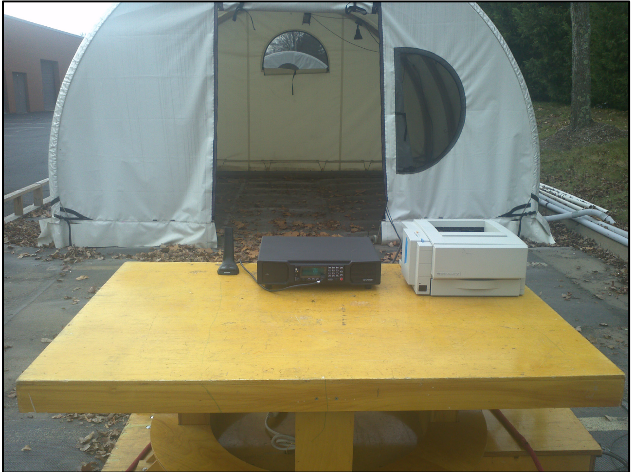
Photograph 1: Radiated Emissions (Spurious/Harmonics) – Front View
