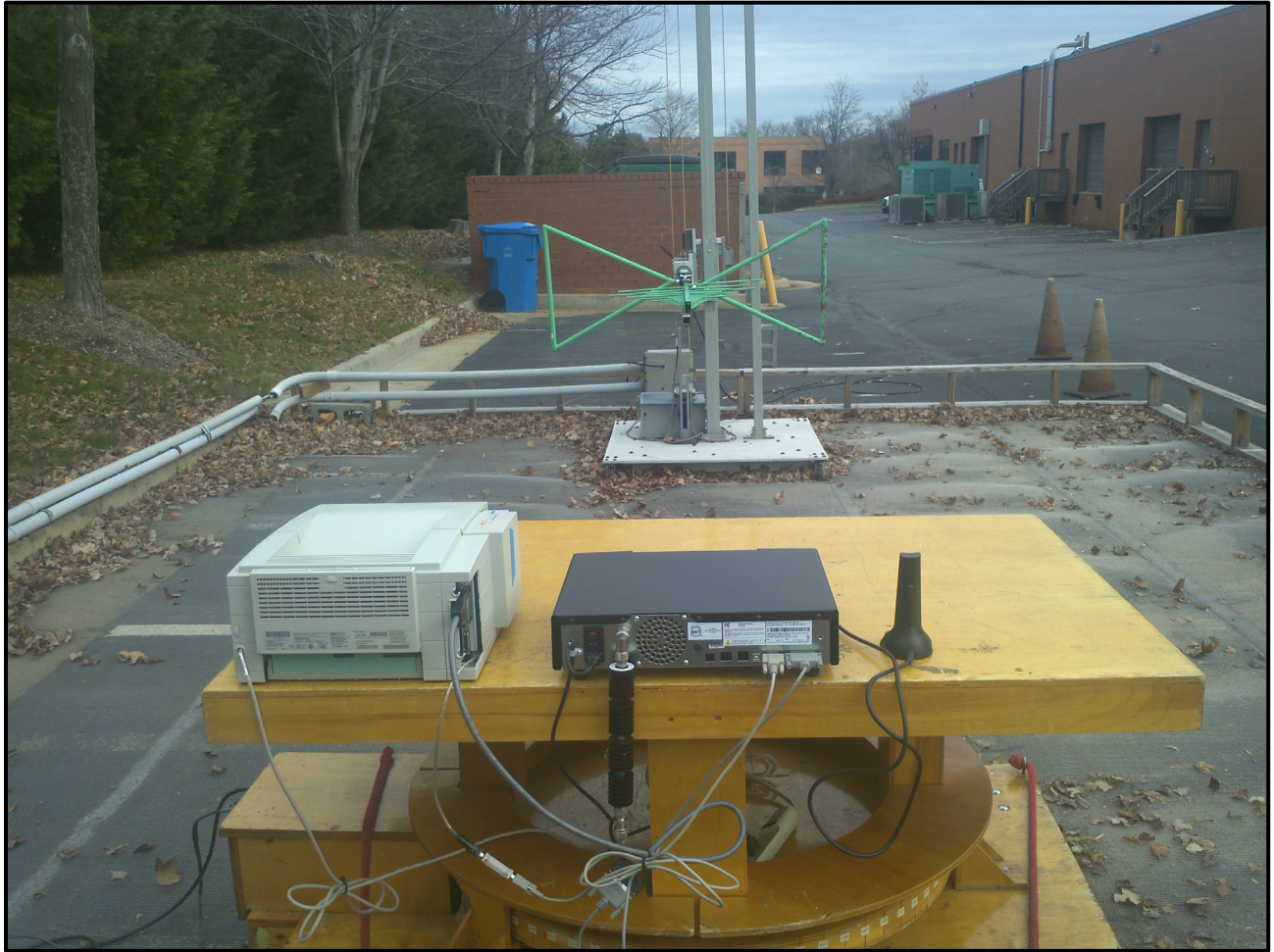
Photograph 2: Radiated Emissions (Spurious/Harmonics) – Back View
