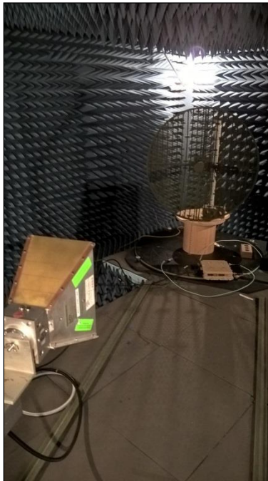
Photograph 6. Undesirable Emissions, 3' Para Above 1 GHz
