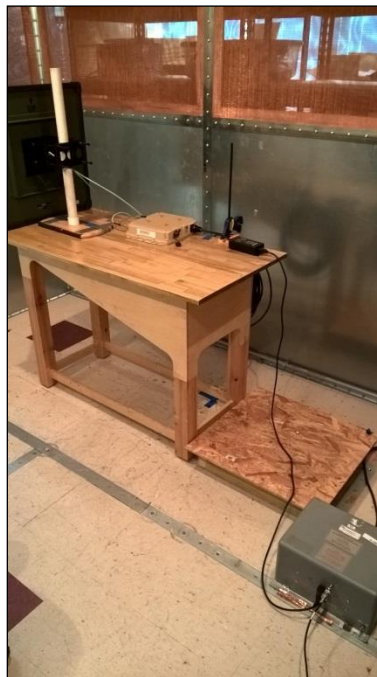
Photograph 14. Conducted Emissions, 2' Panel, Test Setup
