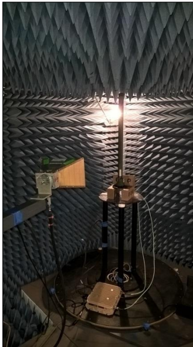
Photograph 10. Undesirable Emissions, 8 Omni Above 1 GHz
