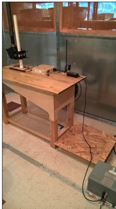
Photograph 16. Conducted Emissions, 5 Omni, Test Setup
