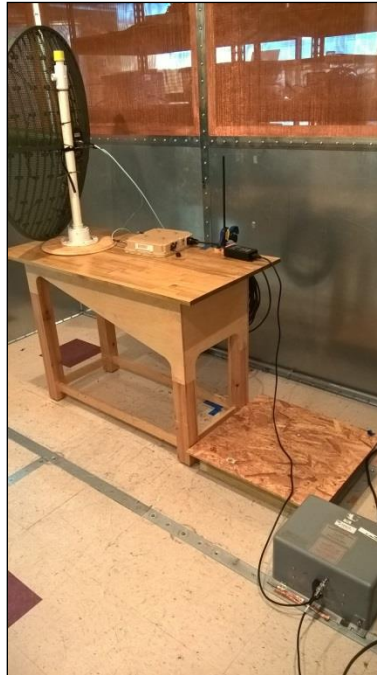
Photograph 15. Conducted Emissions, 3' Para, Test Setup
