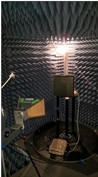
Photograph 2. Undesirable Emissions, 1' Panel Above 1 GHz
