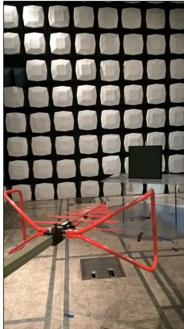
Photograph 3. Undesirable Emissions, 2' Panel Below 1 GHz
