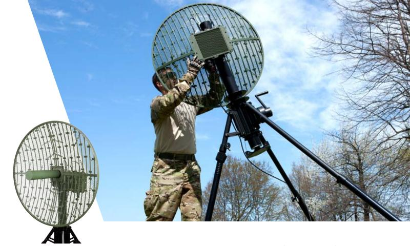
RAPIDLY DEPLOYABLE THREE-FOOT PARABOLIC ANTENNA (4.4 - 5.875 GHZ)
