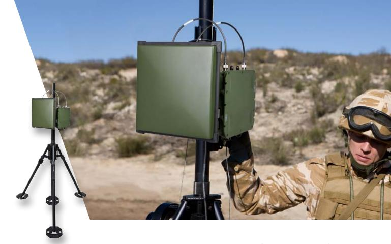
RAPIDLY DEPLOYABLE ONE FOOT PANEL ANTENNA (4.4-5.875 GHZ)
