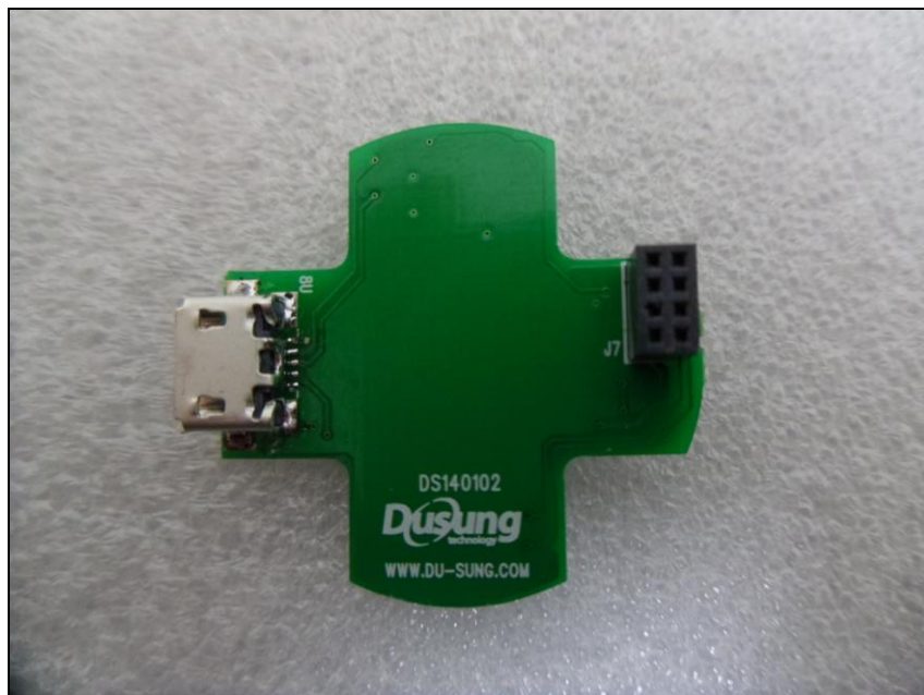
Bottom view of Sub PCB
