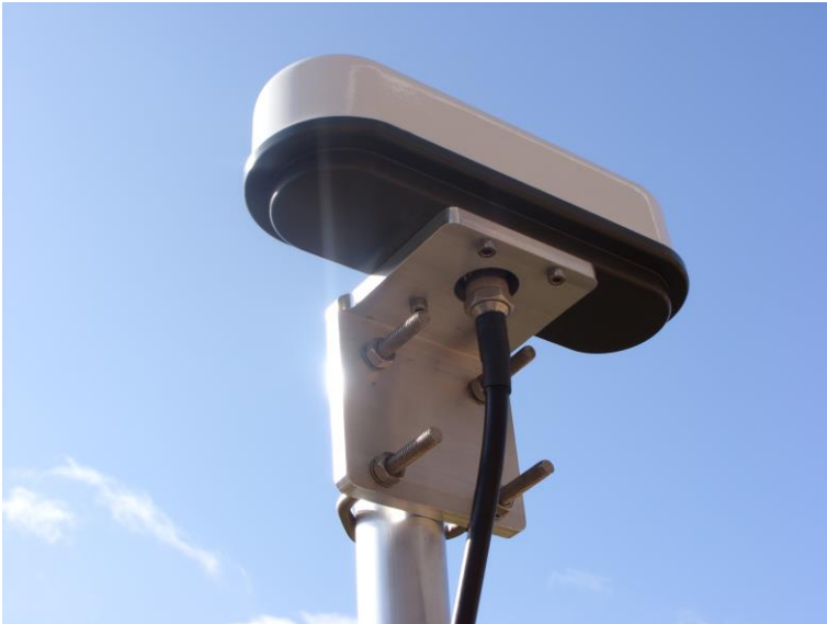
Figure 2. AD511 Active Iridium antenna with mounting bracket and coaxial down-lead
