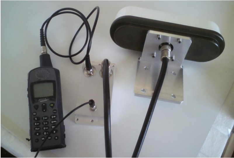
Figure 3. AD510-40 Power Break-In Box for use with +18 to +36 v DC supply.
