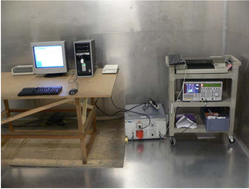
Conducted Emission - Front View
