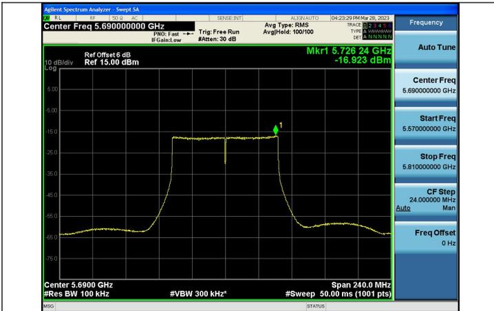
Mode:802.11ac VHT80 Frequency:5690MHz Ant:Chain0
