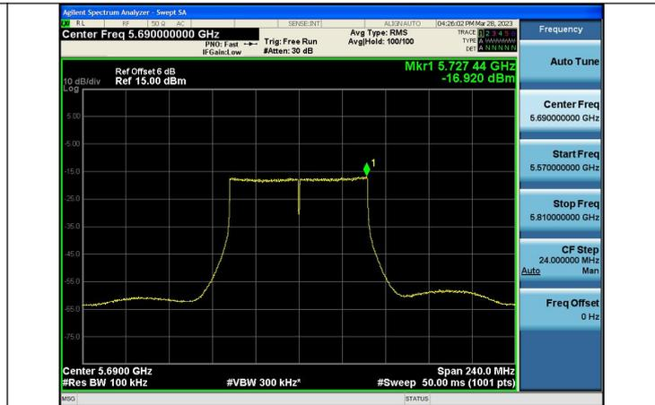
Mode:802.11ac VHT80 Frequency:5690MHz Ant:Chain1
